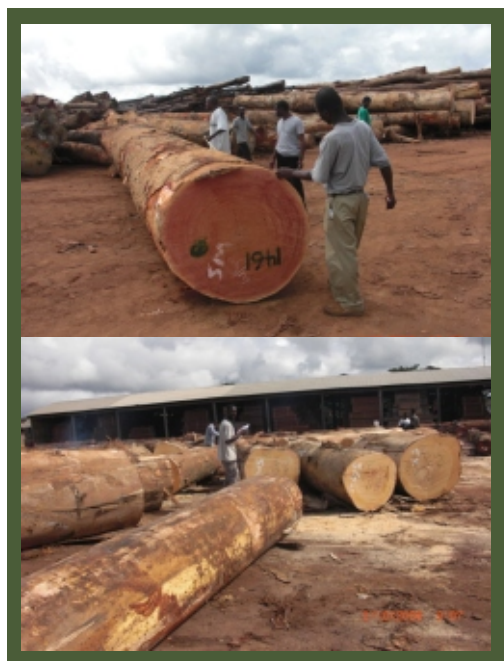
Figure 6: Re-measurement of logs and cutting of bolts for milling
