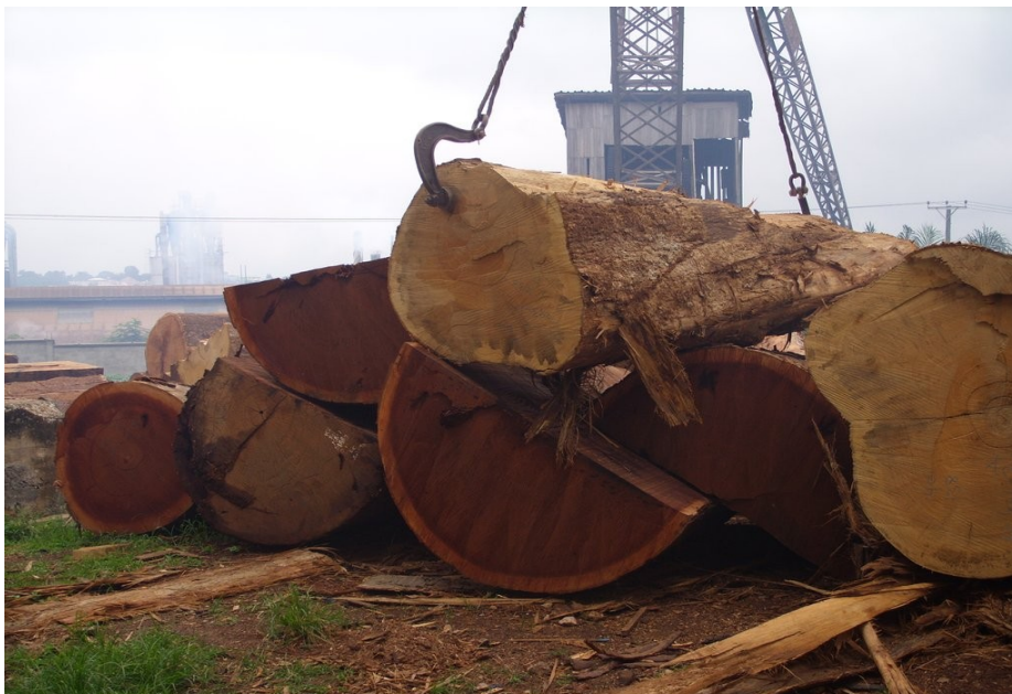
Illustration 9: Log cranes cause limitations in log size and reduce recovery rates. They also are slow as compared to log stackers.
