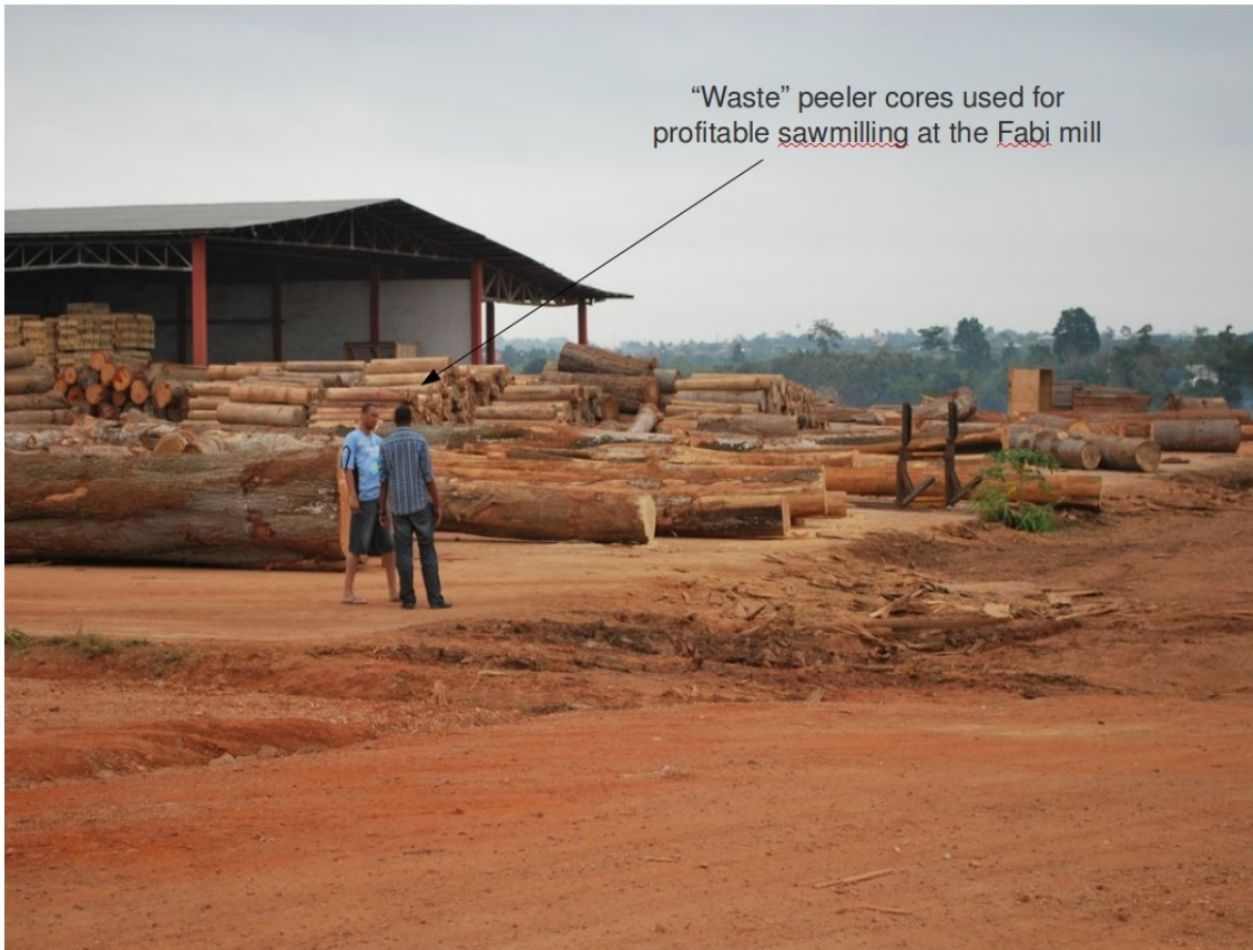
Illustration 2: An efficient sawmill is capable of turning another one's waste into a valuable raw material
