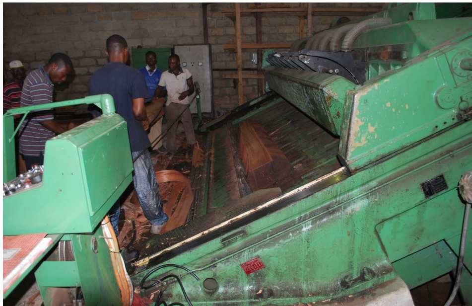
Illustration 5: The workers on this workstation have to remove slice veneer while the machine is operating. This is because there is no system to eject the veneer. The risk is their hands being chopped off.
