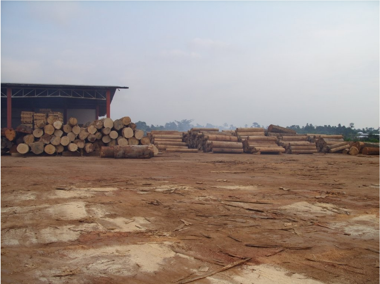
Illustration 10: A paved and clean log-yard is the first step towards doing a good job at cross-cutting, log sorting and log grading
