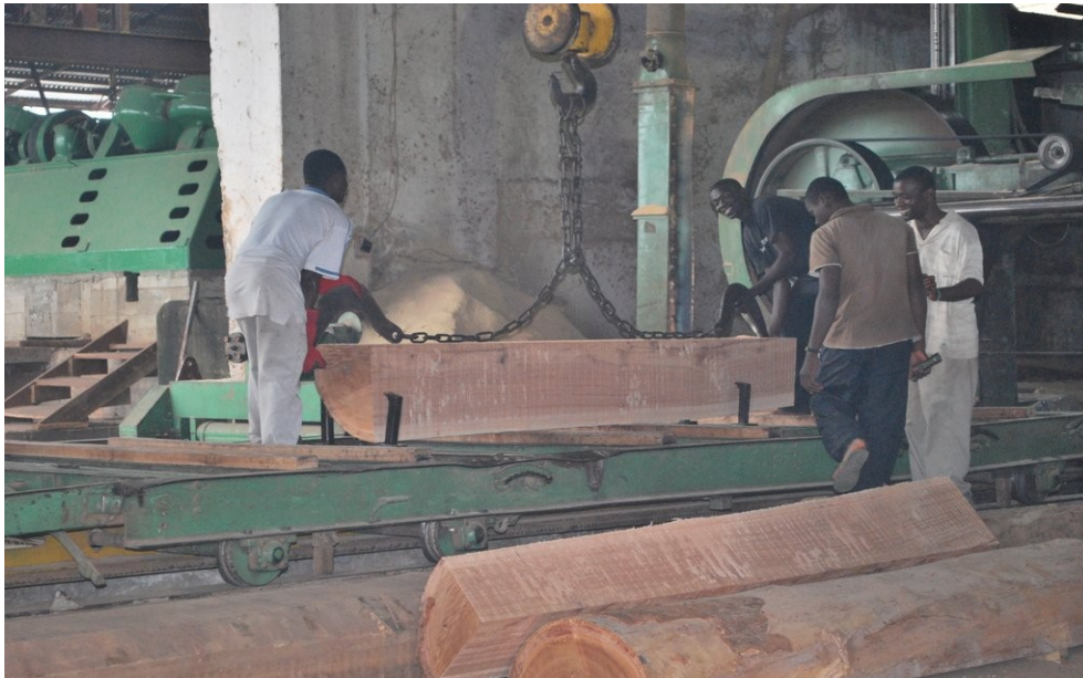
Illustration 4: The band-saw is often running while workers are within a dangerous area
