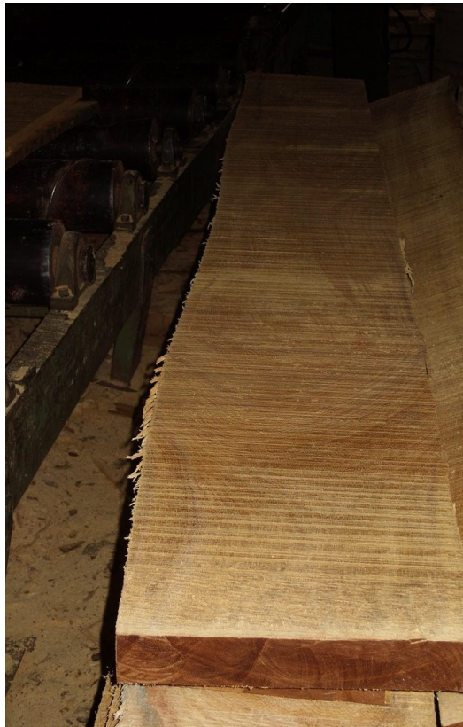
Illustration 1: Imprecise cuts due to poor maintenance and equipment cause heavy losses in Ghanaian wood businesses
