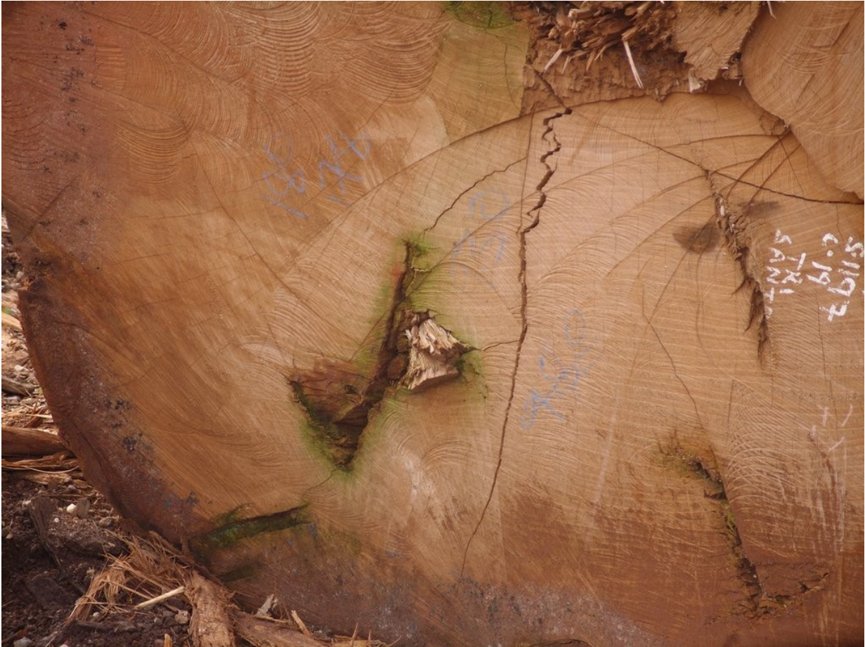
Illustration 11: When there is no record of how long a log is kept in the yard or forest, there is serious risk of downgrading by insect or fungus attack
