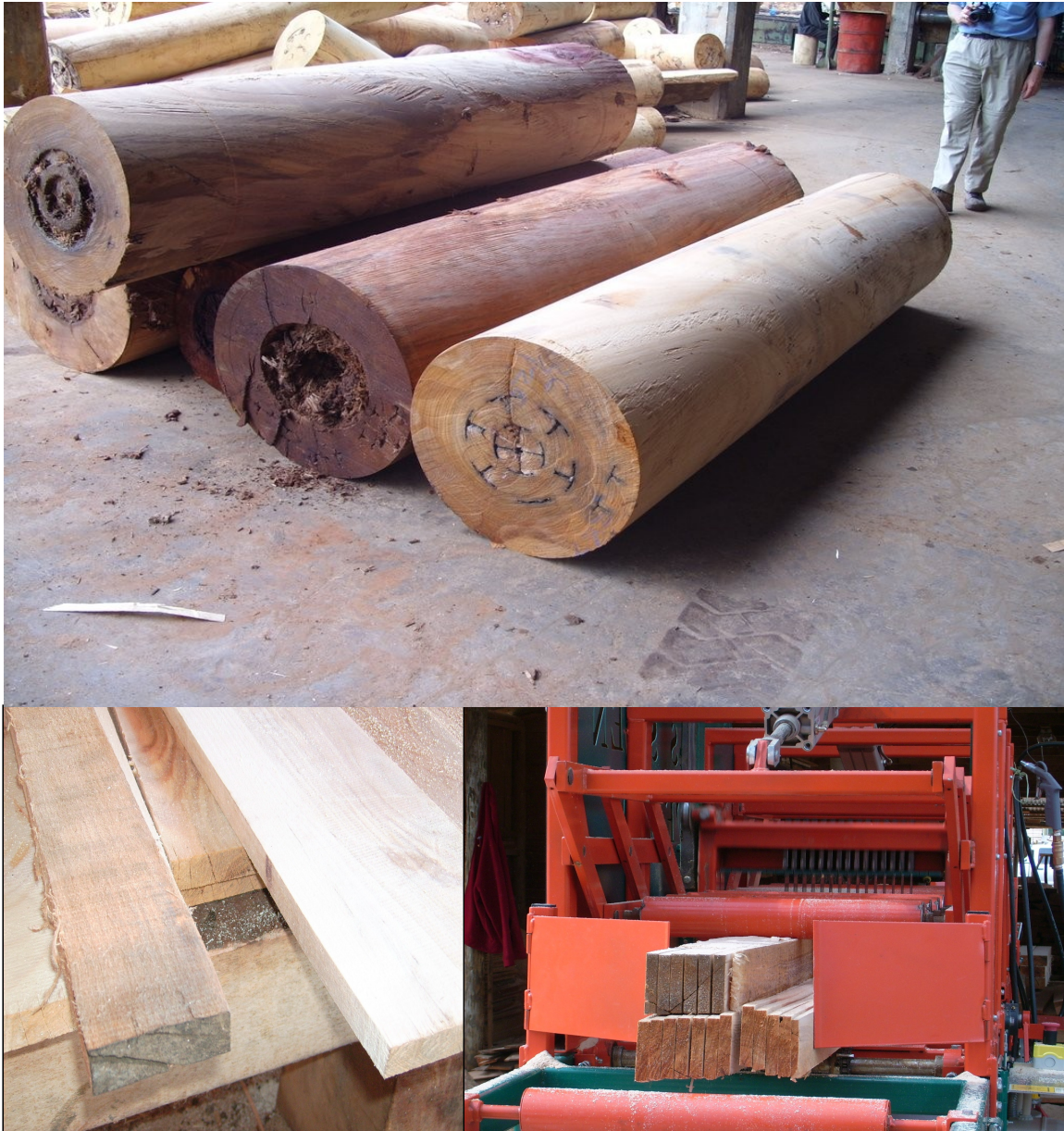
Illustration 15: The Logosol Laks framesaw is a cheap and very efficient way to produce quality small-dimension boards, ideal to use "waste" peeler logs
