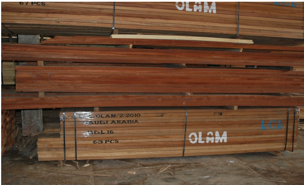
Illustration 3: Poor storage of wood bundles results in hazards for workers, deterioration of products (see bent boards on the picture) and excessive stock-holding.
